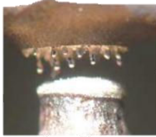
Figure 1 – Image of beading effect on the electrode of an internal combustion engine spark plug
