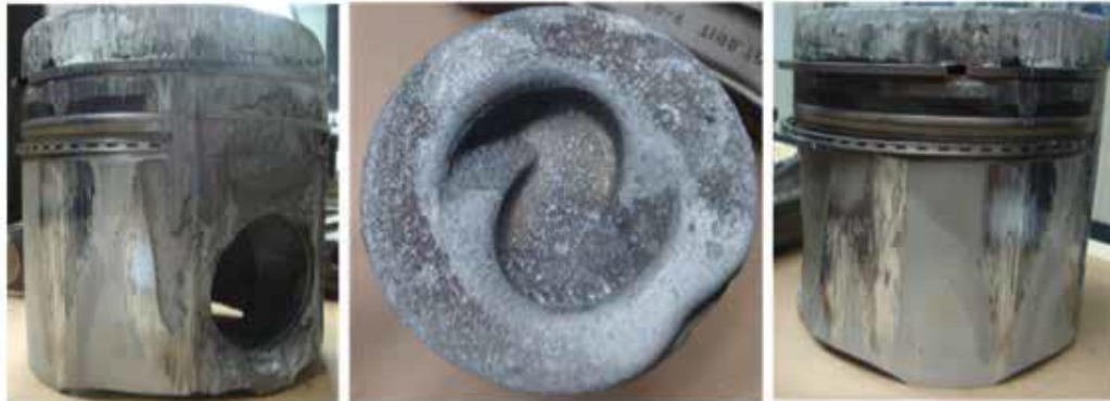
Figure 2 – Piston damage resulting from 300-600 consecutive cycles of engine knock
