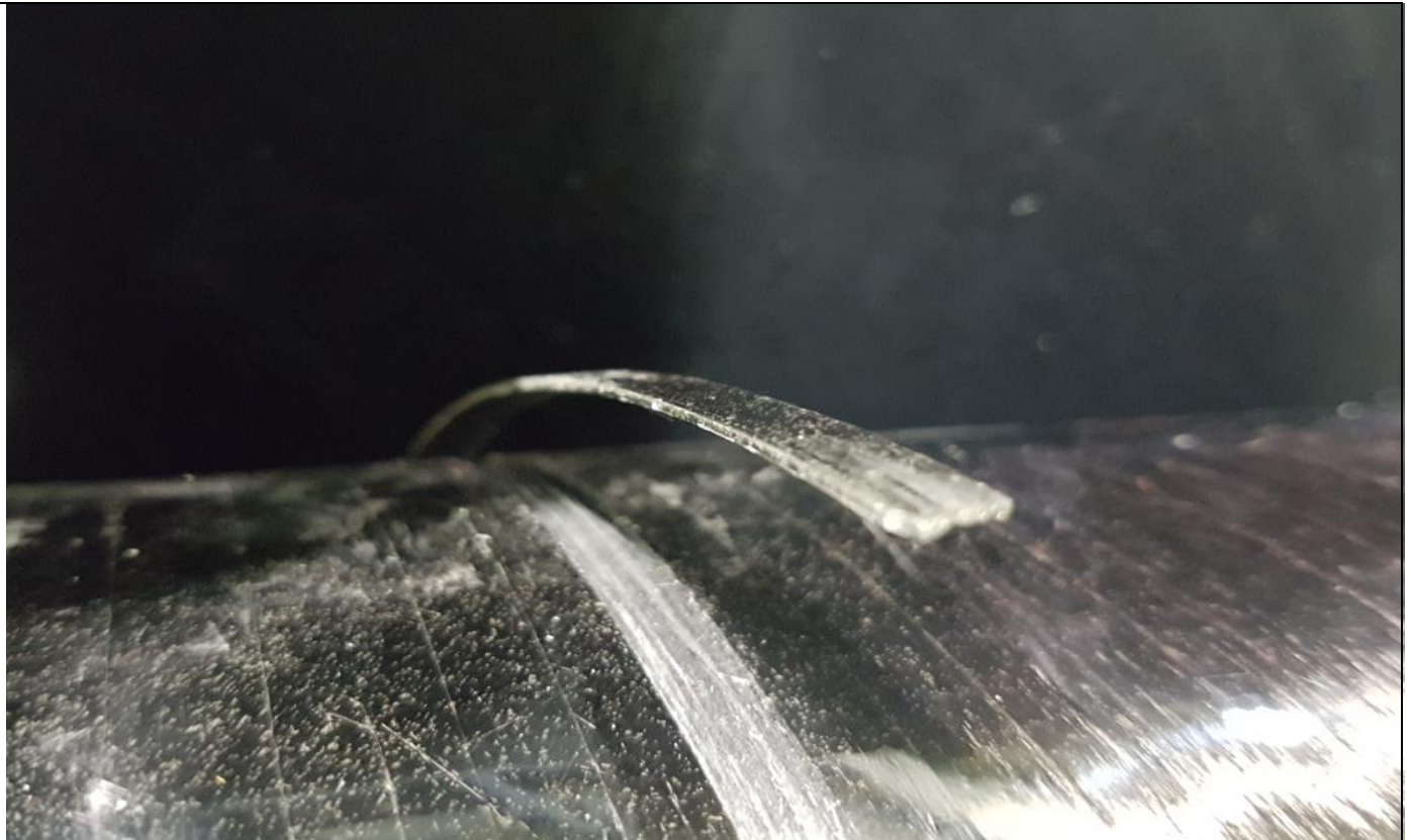
This photo shows the carbon fiber delaminating from the cylinder surface.
