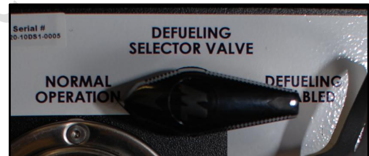
Fuel Module Defueling Selector Valve - Picture Shows Valve Set to Normal Operation
