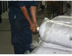
Cylinders should not be handled by Valve / PRD
