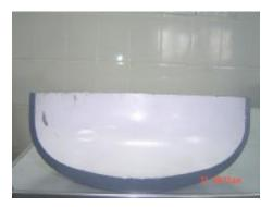
Cut section of type 1 CNG Cylinder bottom
