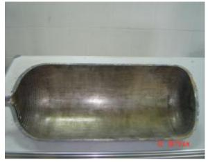
Cut Section of type 1 CNG Cylinder
