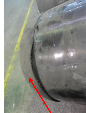
Protection cap remains attached to the dome although the edge is starting to lift. Acceptable
