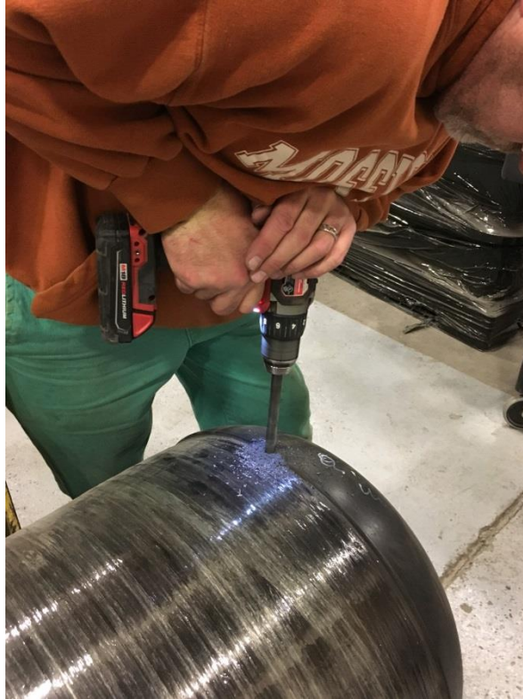
Destruction of the cylinder by drilling a 12mm through hole.
