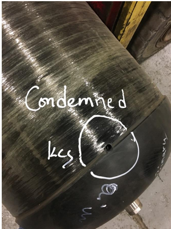
Destroyed cylinder marked as "CONDEMNED".
