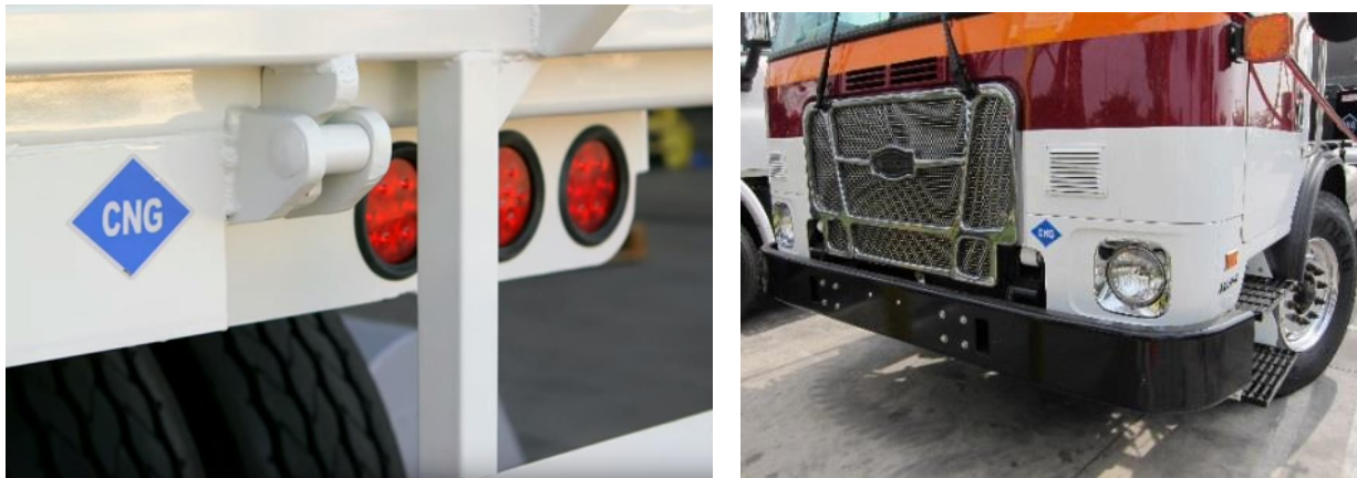
Figure 1 Left: CNG fueled vehicles are identified by a blue and white decal on the right rear of the vehicle. Right: A CNG decal may also be on the left front of the vehicle as shown.
