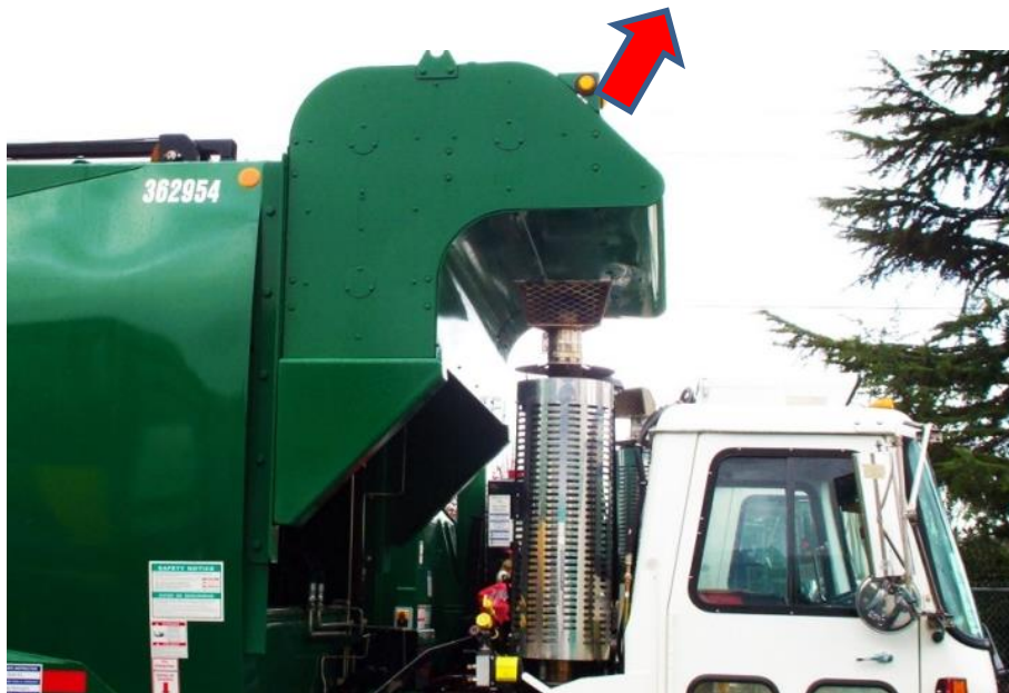
Figure 7 CNG PRD venting locations and direction, front of body refuse system.
