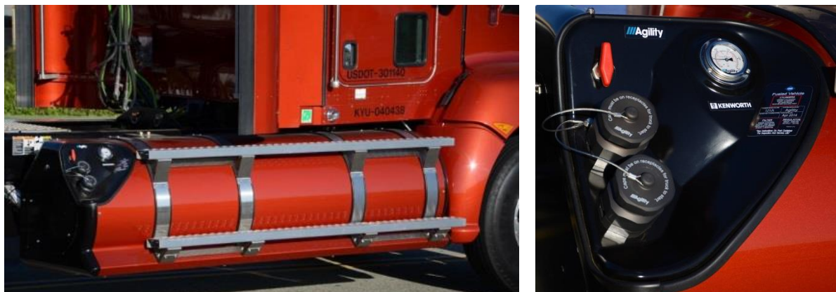
Figure 10 CNG FMM mounted on a side mount system.
