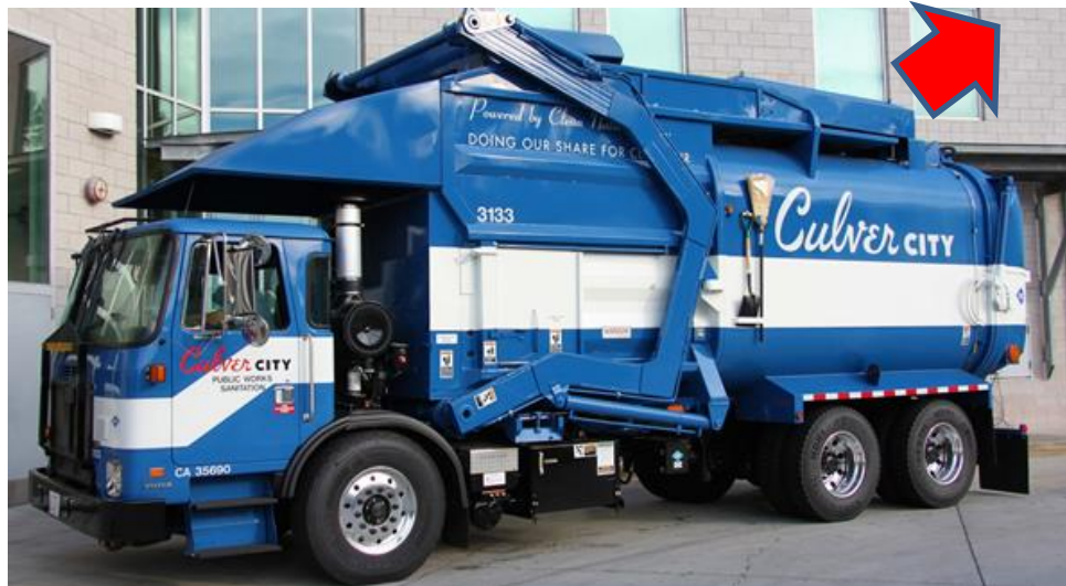
Figure 5 CNG PRD venting locations and direction, refuse roof mount systems.
