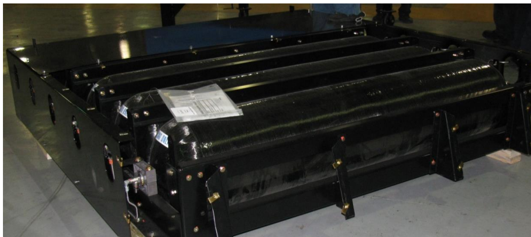
Figure 4 Five Type 3 or Type 4 CNG cylinders reside inside the housing. PRDs are located at each manual valve and centered along the length of the cylinder for a total of 10 PRD and vent locations.
