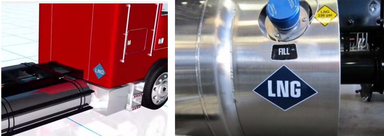
Figure 11 Left: LNG blue diamond decal location at the lower right rear of the cab on vehicles without bodies such as a roll-off refuse hauler. Right: LNG decal on the right end of the fuel tank.
