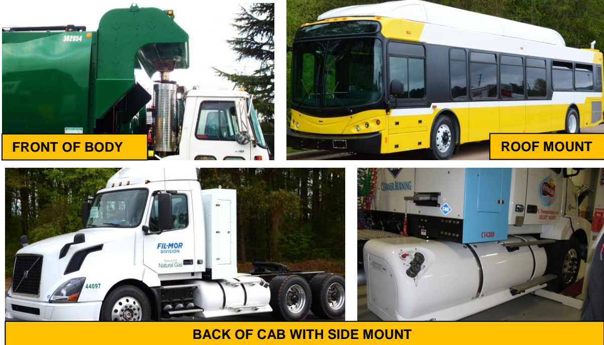
Figure 2 Popular CNG fuel system configurations offered by Agility Fuel Solutions.
