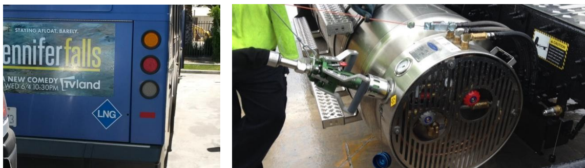
Figure 12 Left: LNG decal on the right rear of a transit bus. Right: The “valve end” of an LNG fuel tank.
