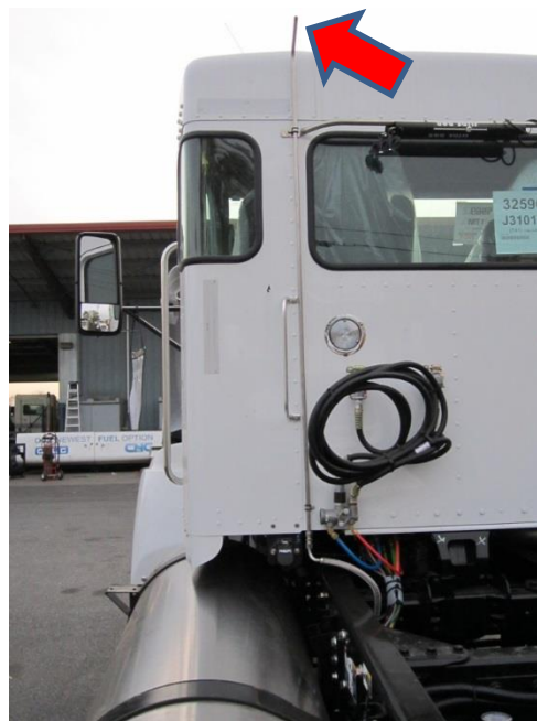
Figure 14 LNG vehicle, rear view. The LNG tank is on the lower left and the vent line runs from the tank and up the rear of the cab, terminating above the cab. LNG vent tubes look like their CNG counterparts – but beware that LNG vehicles may vent in normal operation. See text for more details.
