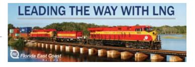
In November, the Florida East Coast Railway unveiled its modified fleet of 24 GE ES44AC locomotives, which operate in pairs with a purpose-built fuel tender supplied by NGVA member company Chart Industries. The EPA Tier 3-compliant locomotives look identical to standard ES44ACs, but their GEVO prime-movers have been retrofitted by GE with its NextFuel low-pressure technology, giving the railway the flexibility to run on both diesel fuel and LNG with up to 80% gas substitution or 100% diesel.
