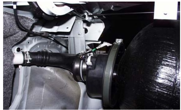
Figure 4.4 Formed vent cover (L. DaShiell)
